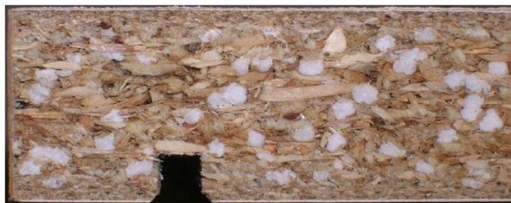
Figure 5: NAV LiteBoard 16mm, cross-section with cut groove
