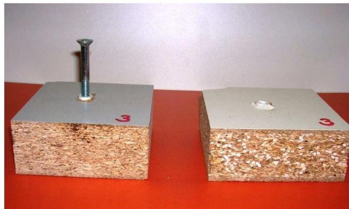
Figure 3: Glue-in thread insert after extraction tests in normal particle board and NAV LiteBoard
