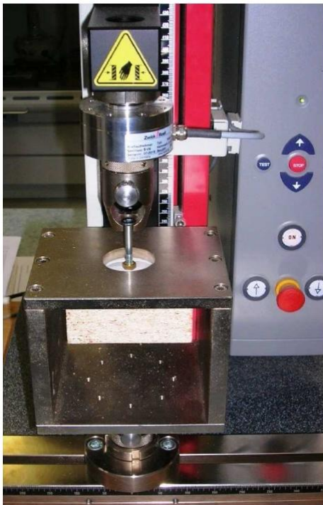
Figure 2: Test design: Extraction of an extraction anchor
